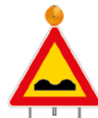
FIG. 389 ART. 31 STRADA DEFORMATA
